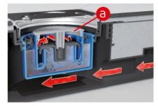
Overpressure in the sewer: The valve disc is pressed against the valve seat, so no smell may get out. A further advantage: the trap is save against back flow.
