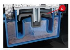
When the water from the shower runs throuth the trap, the valve disc opens.
