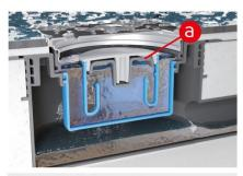
When the valve disc is opened, the water may pass the trap as usual.
