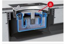
if the water inflow is stopped, the valve disc closes, the water stays inside the trap.
