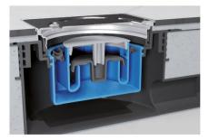
Should the water inside the trap be evaporated, e.g. caused by a floor heating, the mechanic trap protects from bad smell
