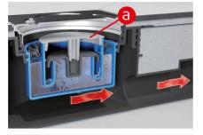
Underpressure from the sewer: The weight of the valve disc together with the water inside the trap protects from getting sucked out.
