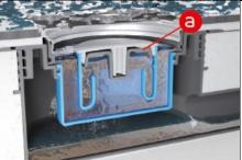
When the valve plate (a) is opened, the water can flow unhindered
